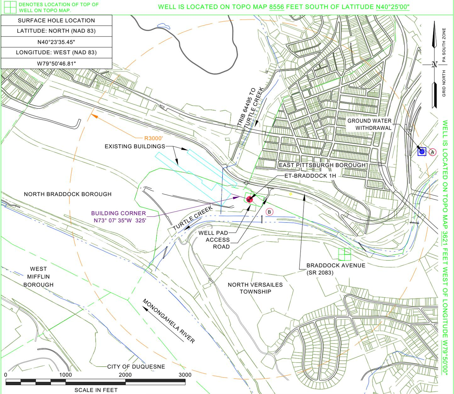
THIS PLAN IS FOR WELL LOCATION PURPOSES AND IS NOT A BOUNDARY RETRACEMENT SURVEY. TIES TO SURVEYED MONUMENTS ARE FOR GAS WELL RE-LOCATION ONLY.
