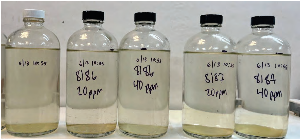
6/13/24 - Nalco 8186 & 8187 Coagulant Testing
