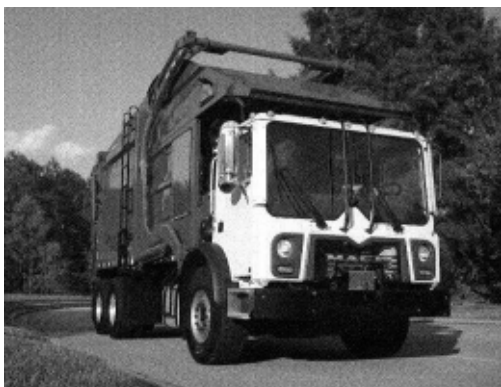
Figure 1-2 Top 10 2017 Mack 40 cubic yard Front Loading Recycling Truck
