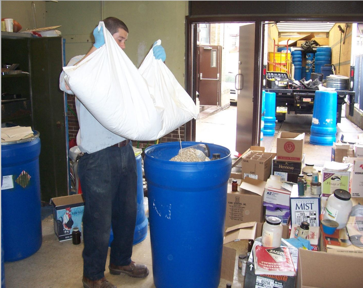
Disposal contractor (PSC) pouring a spill control absorbent (vermiculite) into a 60-gallon disposal drum
