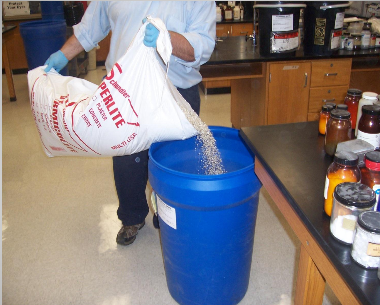
Disposal contractor (PSC) pouring a spill control absorbent (vermiculite) into a 30-gallon disposal drum
