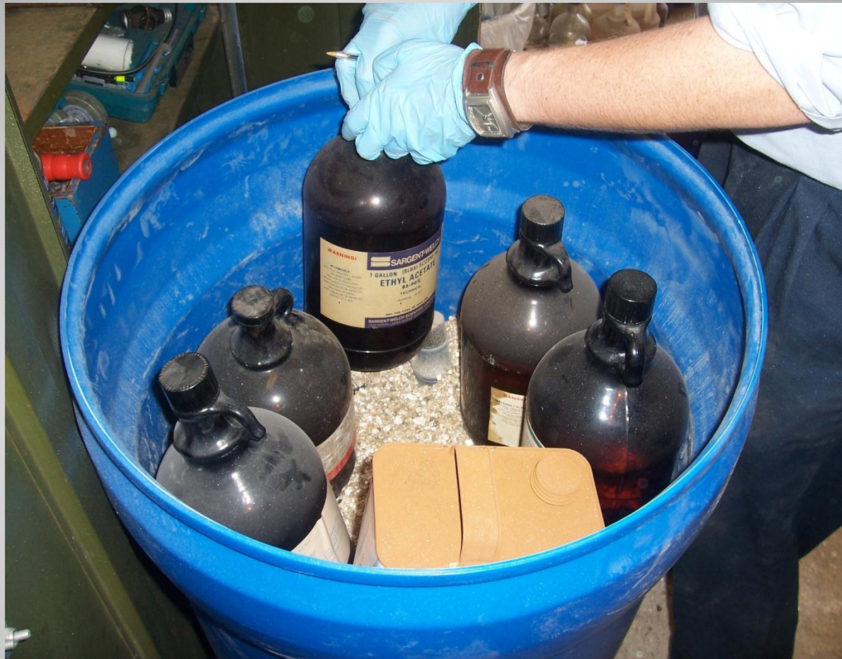
Disposal contractor (PSC) placing flammable liquids into a 60-gallon disposal drum
