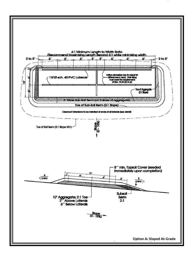
4:1 Minimum Length to Width Ratio 6' 6' 6' 2 to 5' 6' 3' 2 to 5' 6' 3' 6' ò S 3 - 11/2"Ø sch. 40 PVC Laterals 0 W Ø Onlices -al-A 0 (2:1 Sope) Cleanout Extensions to be installed at ends of all laterals (see detail) Sope - 15%) Toe of Soll Berm (3:1 Slope Min) -12" min. Topsoll Cover (seeded Immediately upon completion) w 3 1 (min) 2 to 5' 6' 2 to 5 3 (min) 1 10" Aggregate; 2:1 Toe-2" Above Laterals 6" Min Below 10-15 Option B: 'Level At-Grade'
