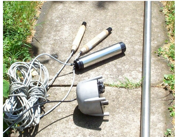
Figure F.2: ORP, pH, DO, and Sonatex Probes
