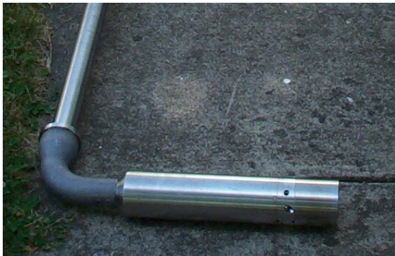
Figure F.3: At low level, some instruments are above surface. Sludge blanket interface probe at lower right.
