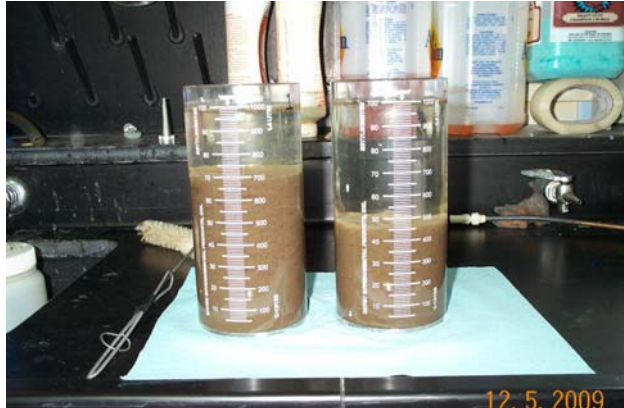
Figure D-8: Sludge Settleability Tests at 30 min, 5/12/09
