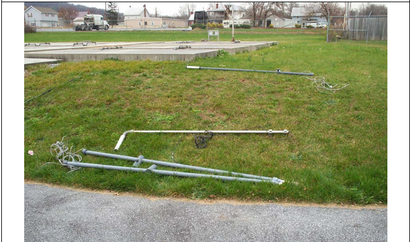
Figure F-2: Probes affixed to mounting poles (top to bottom: DO, NO3, ORP, pH/Temp).
