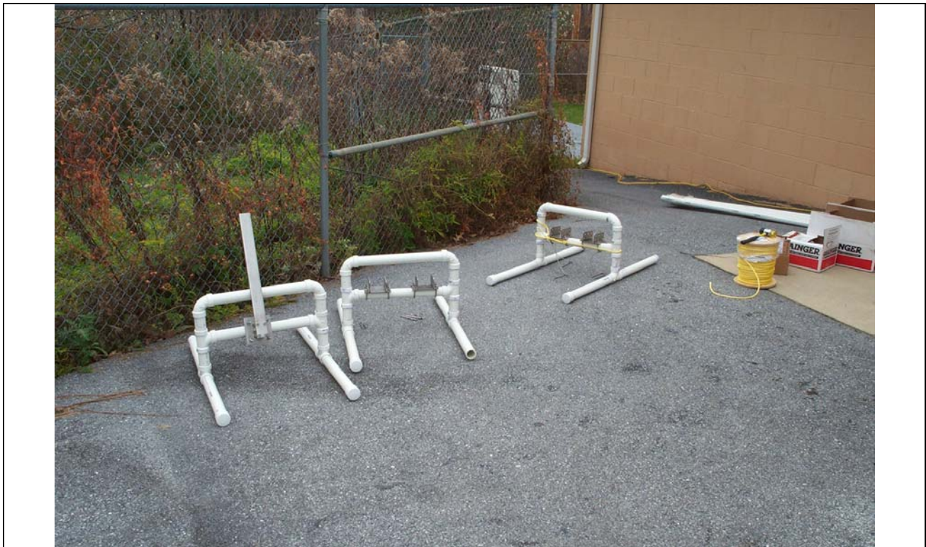
Figure F-1: Probe mount stands fabricated from Schedule 40 PVC pipe.
