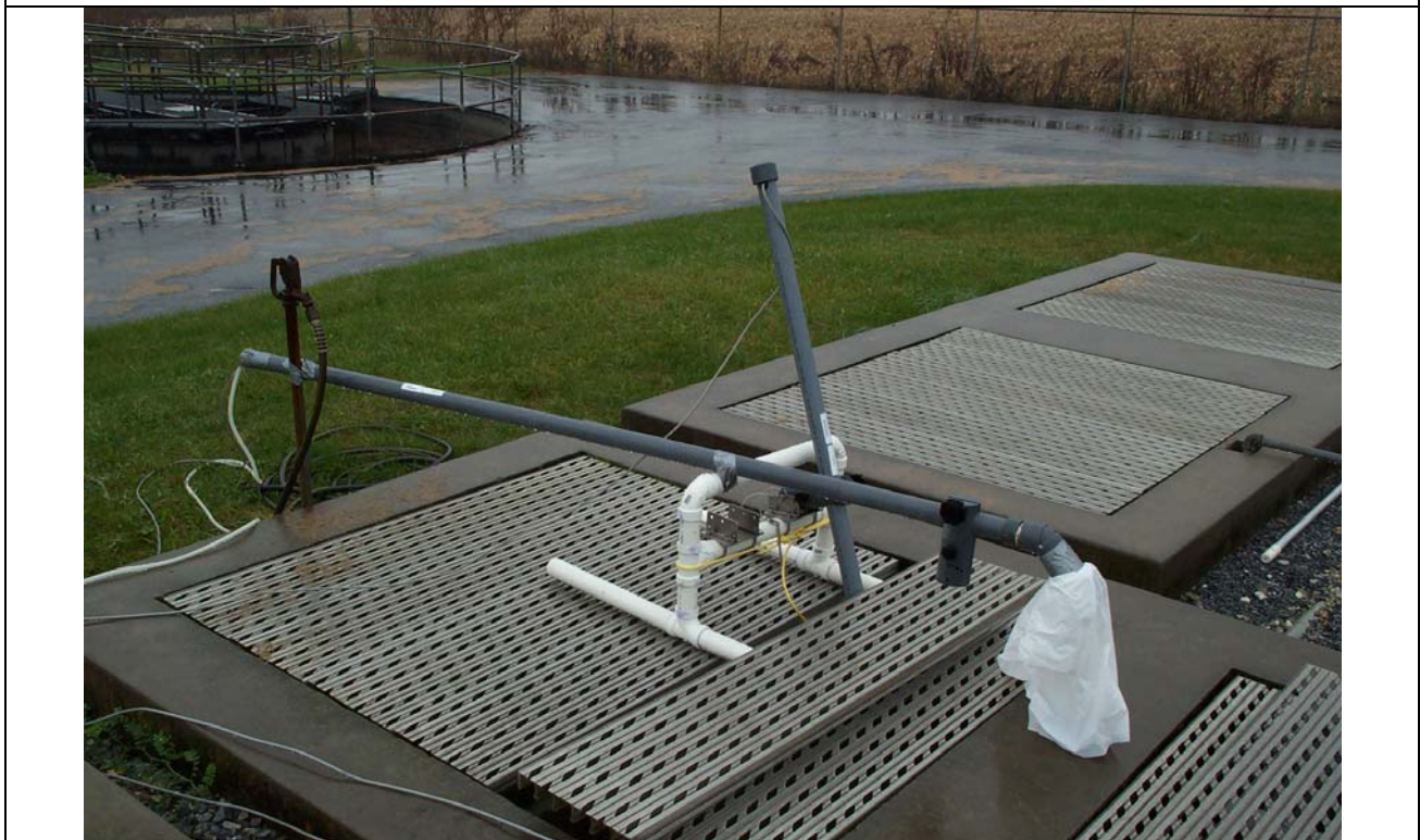
Figure F-4: Ammonia probe being calibrated overnight using standard solution.
