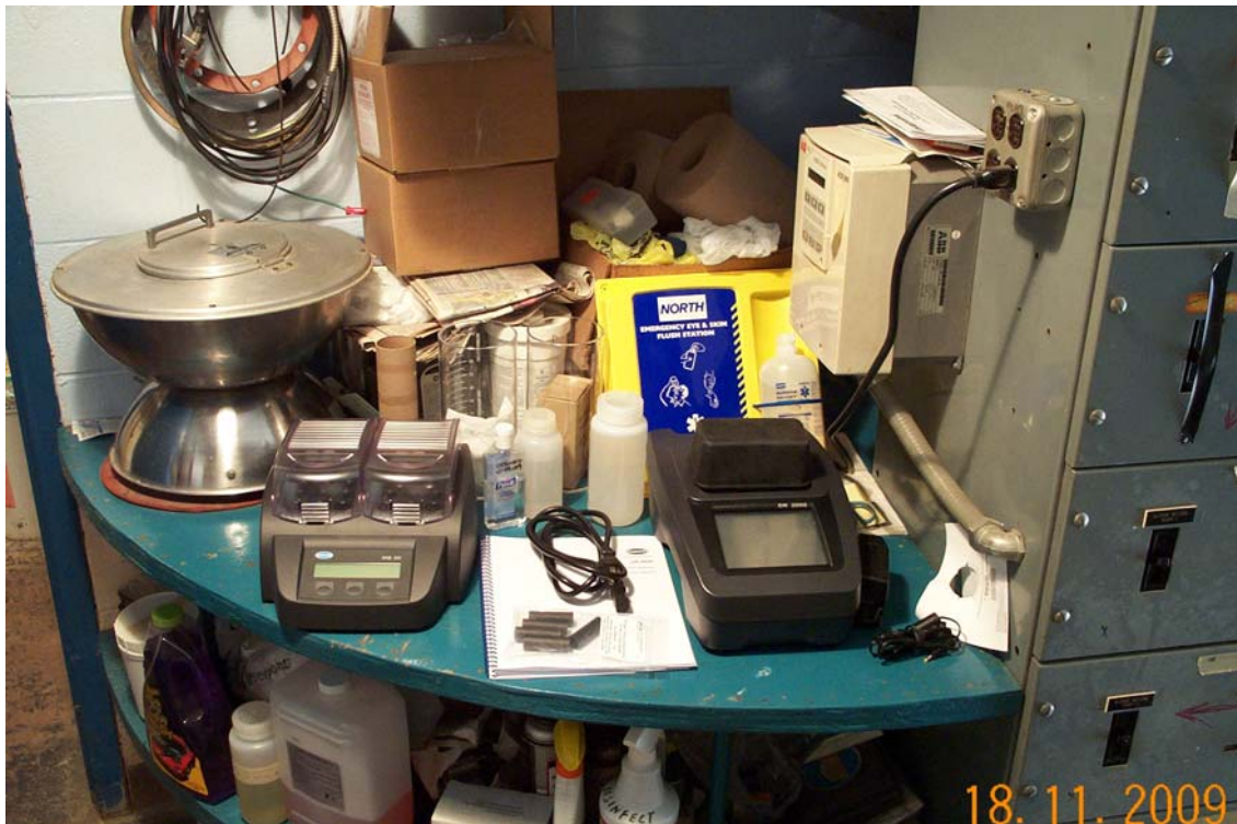
Figure 35. Centrifuge, heater block, DR2800 setup area
