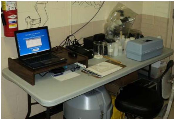
Figure G-14: WPPE Bench with SCADA recorder
