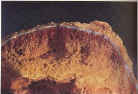
FIGURE 2-21. Scale With Enveloping, Shell-like Layer (Unfavorable conditions), Filamentous Structures of Iron Bacteria
