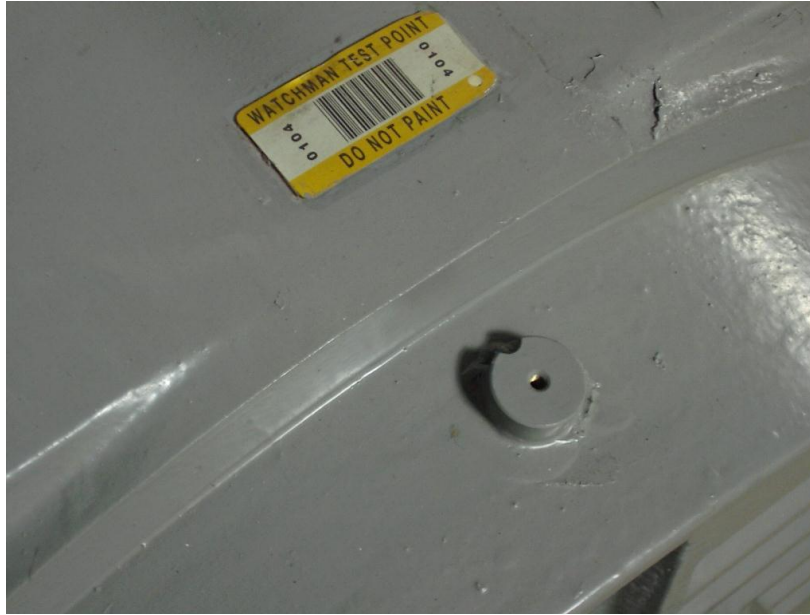
Figure 3.2 Vibration Analysis Point
