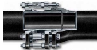
Figure 2.5 – Mechanical Coupling Joint 4
