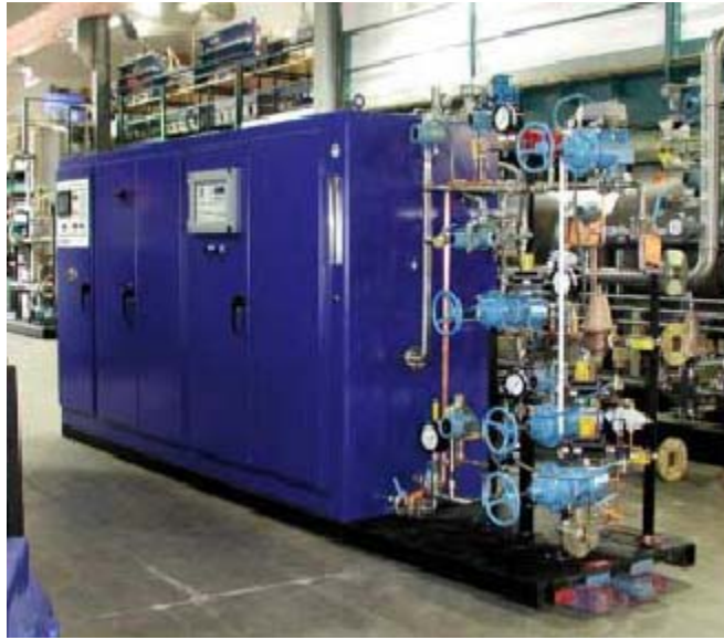
Figure 2.3 – Ozone Generator Power Supply Unit 1
