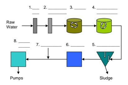
A clear well allows the treatment plant to operate at a \_\_\_\_\_\_ rate, building up reserves during low-use hours and maintaining supply during peak-use hours.
