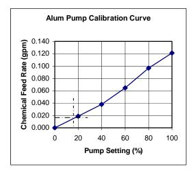
Ans: [Chemical feed rate = 0.014 gal/min → Feed Pump Setting = 14%]
