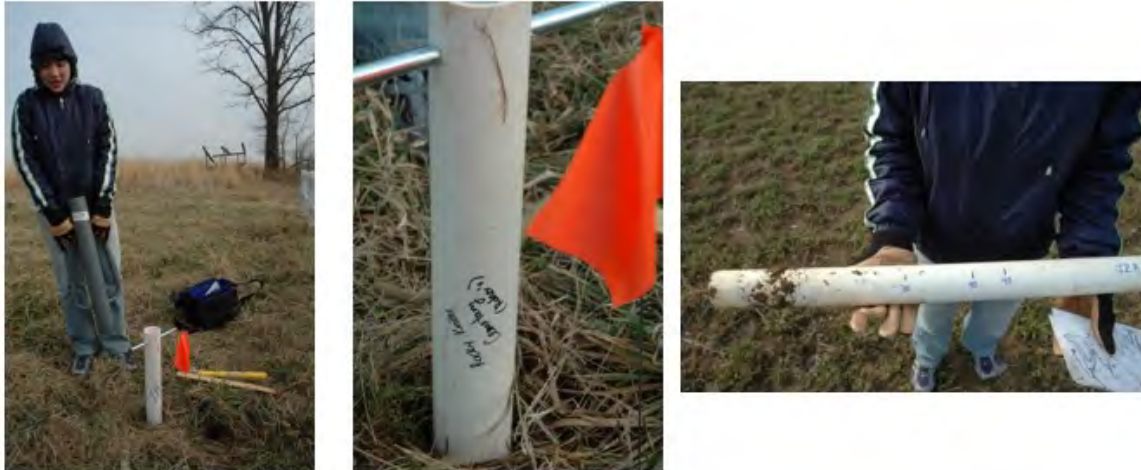
Figure E.2.3 Alexandra Sullivan (F&M '06) collects core samples at the BSR reference site, an 18 th Century cemetery on a knoll overlooking the BSR watershed. A fence-post driver is used to pound a sharpened PVC tube into the soil, to a depth of 45 cm. This depth is presumed to be below the influence of 137 Cs deposition.
