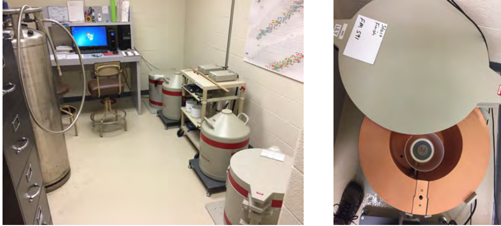
Figure E.2.5 Franklin and Marshall College gamma spectroscopy laboratory, funded by the U.S. National Science Foundation (NSF-MRI NSF-MRI 0923224), with support from PA DEP.: (Left) Two lead-shielded detectors and two liquid nitrogen dewars line the right side of the lab. The multichannel analyzers are on the small table between the detectors; (Right) View into a copper coated, lead-shielded detector with a sample in place for analysis. The sample rests on the base of a 1L plastic Marinelli beaker that fits over the detector window. A PVC spacer prevents the Marinelli beaker from touching the detector.
