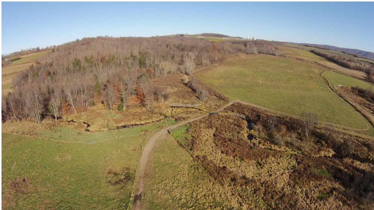
Stream corridor rehabilitation project located within Alba Creek, Bradford County and 1,800' of additional tributaries. Project consisted of riparian buffer, streambank fencing, and streambank rehabilitation. (2012)
