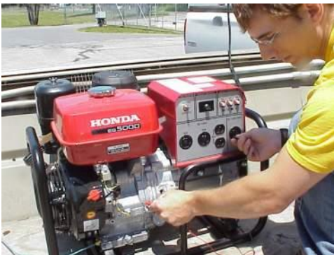
Pic. 7 – continuity check between power receptacle contacts And generator. (NO continuity)
