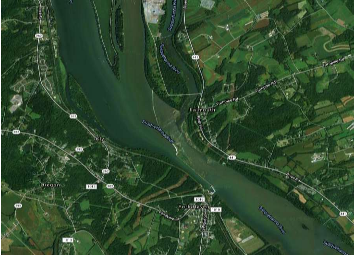
Figure 1-4. Imagery of the impoundment at York Haven, PA illustrating the constriction and mixing of the water quality influences between Rockville and Marietta. This impoundment is somewhat unique in that it not only pools the water, which allows for mixing, but it forces the release of water unevenly in the lateral (across the width of the river) scale.
