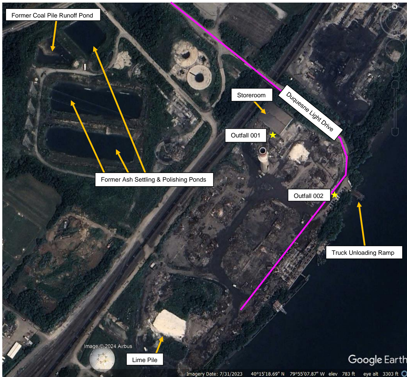
Figure 1. Current points of interest shown on outdated satellite imagery of partially demolished power plant
