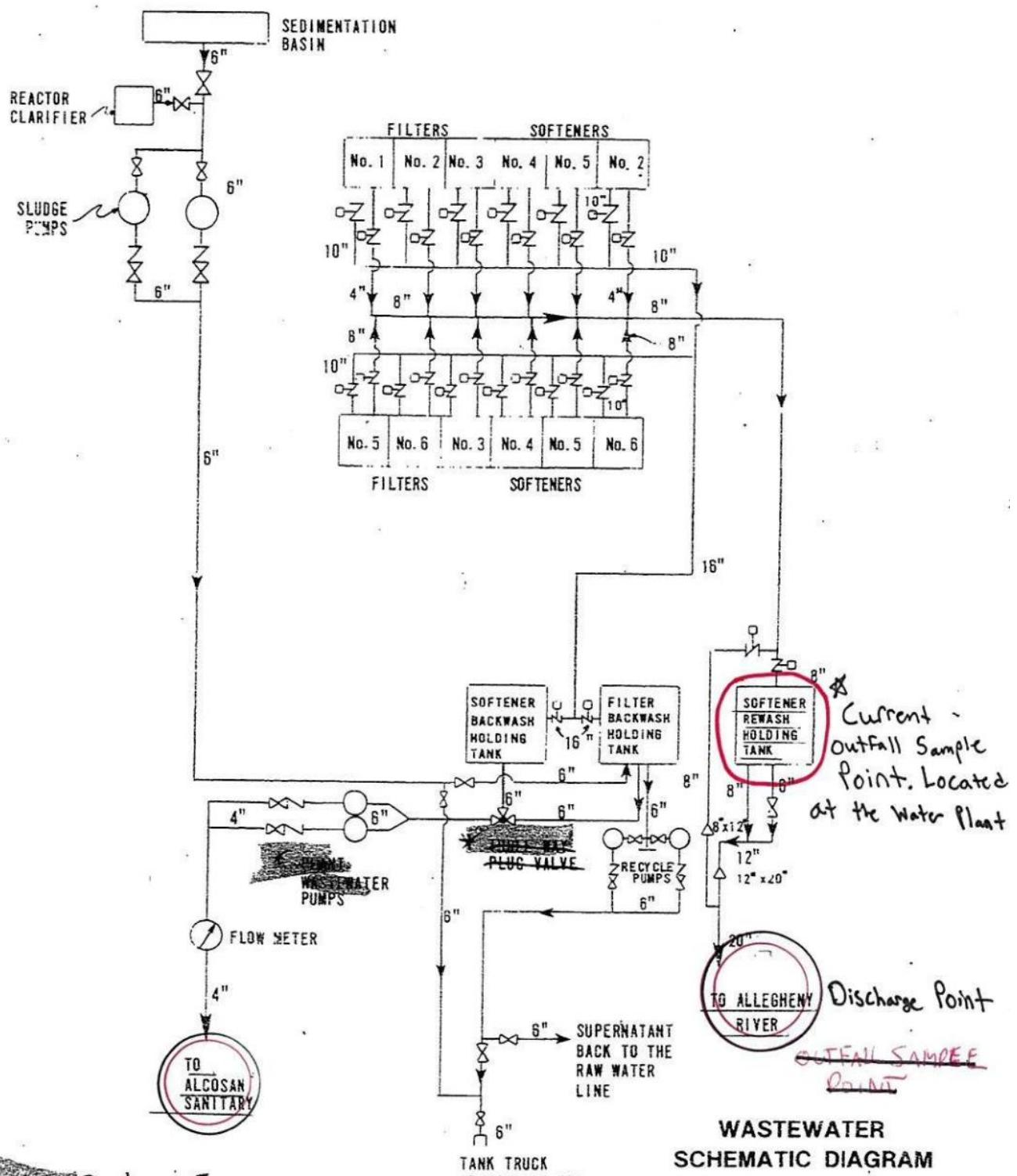
WASTEWATER SCHEMATIC DIAGRAM
