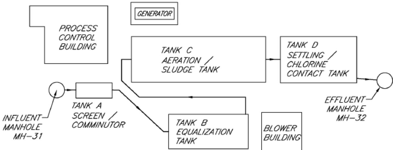
Existing tanks B, C, and D will be removed. Existing pumps, blowers, and process piping associated with these structures will also be removed. The influent manhole, effluent manhole, and standby generators are proposed to be retained and reused. Process control and blowers will be removed from the existing buildings. The buildings are proposed to be retained for non-treatment uses.
