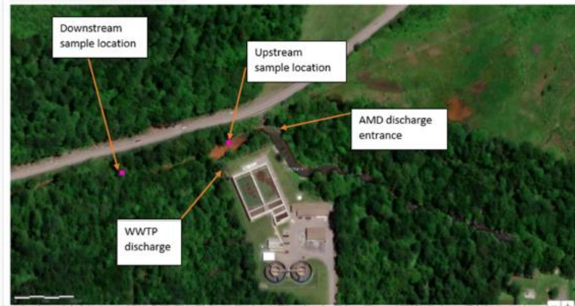
Figure 2. Map of Portage Area Sewage Authority Wastewater Treatment Plant, sampling locations, and Little Conemaugh River.
