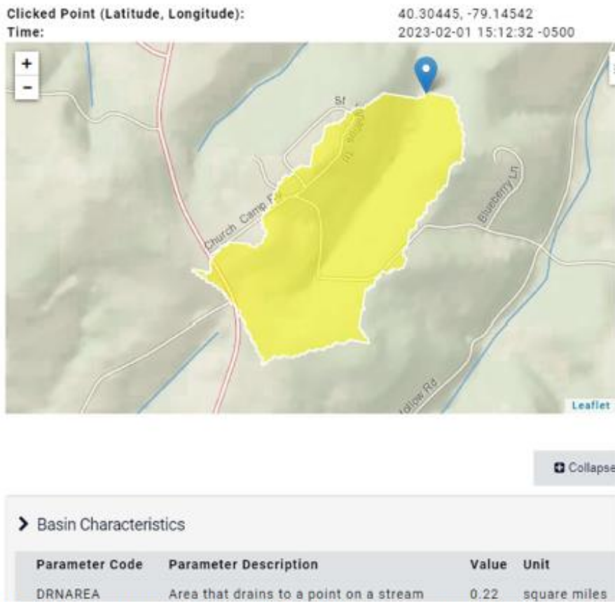
Figure 3. USGS StreamStats report for the drainage area to the POFU survey location.
