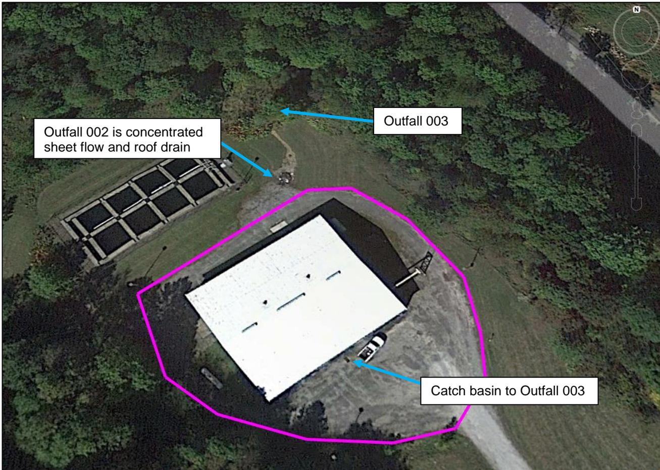
Figure 2. Sugar Run Water Treatment Plant with stormwater drainage area shown in pink
