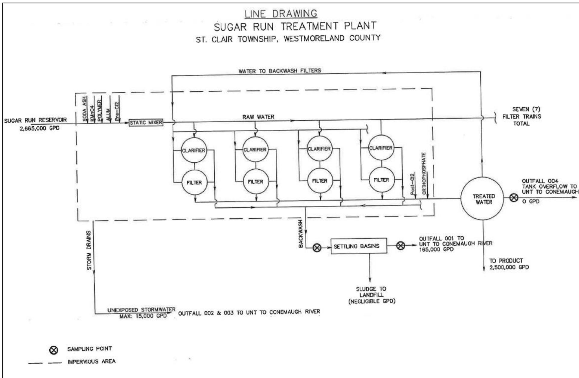
Figure 1. Line drawing of Sugar Run Water Treatment Plant
