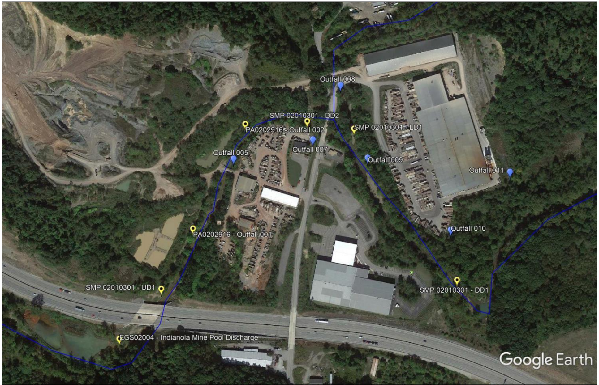
Figure 1. Aerial View of the Harmar Plant with PA0253570 Outfalls (Blue) & SMP 02010301/NPDES PA0202916 Monitoring Points/Outfalls (Yellow)
