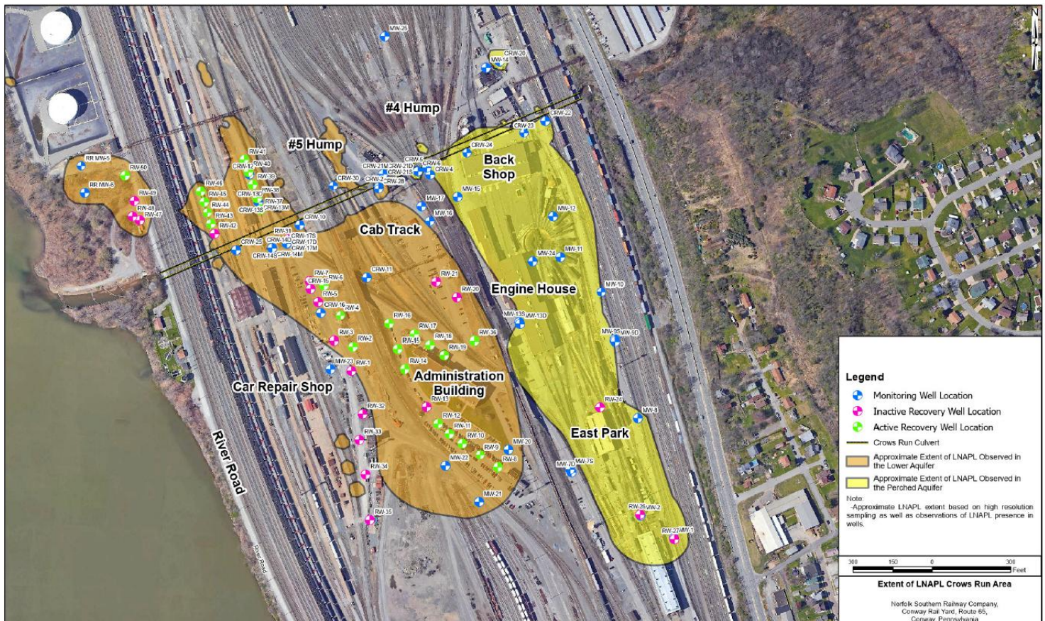
Figure 2: LNAPL Contaminated Aquifers Below Conway Railyard January 2025
