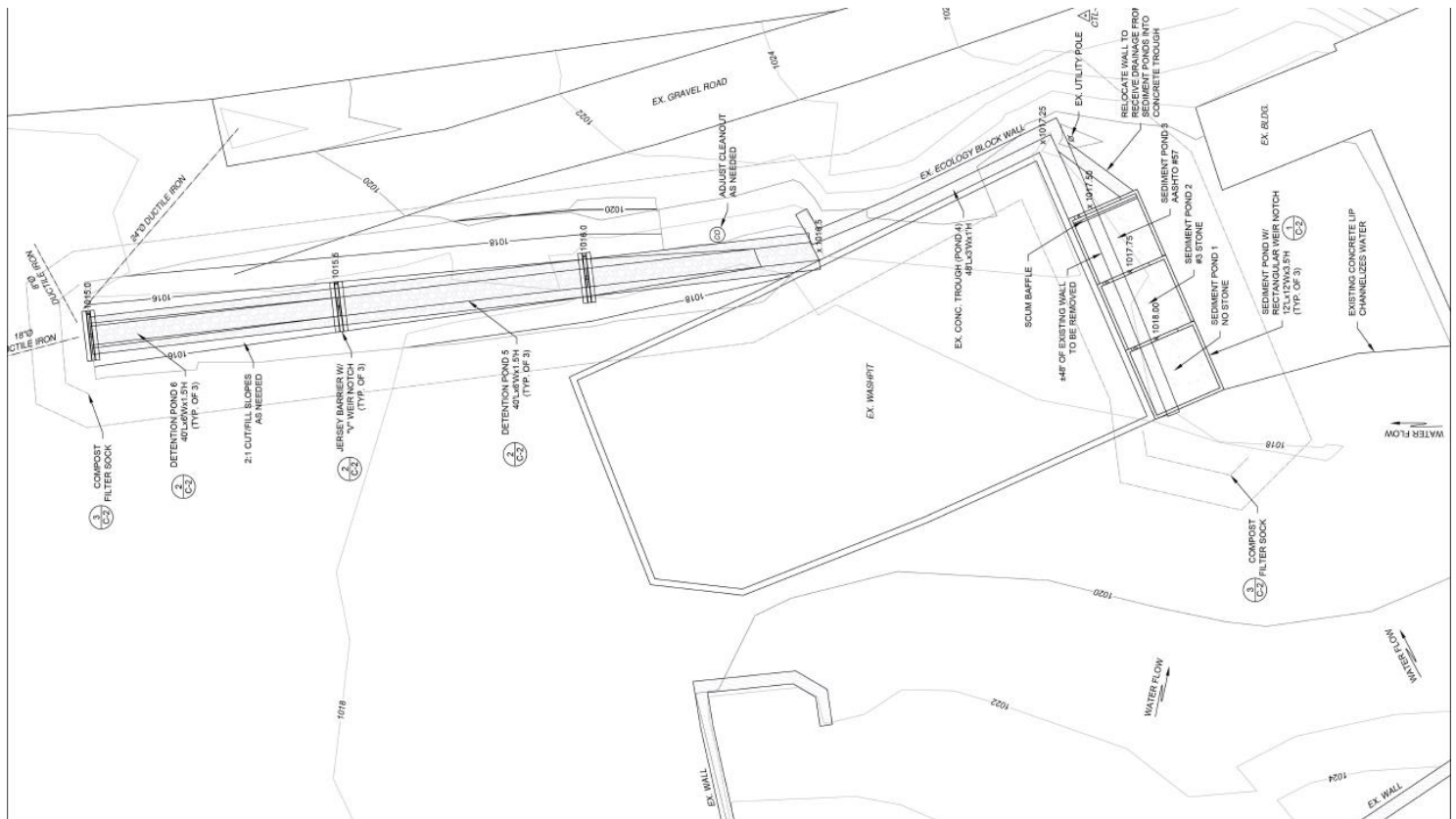
Figure 1: Marcon Hopwood Washout, 3-Sedimentation Ponds and 3-Tiered Detention Pond System
