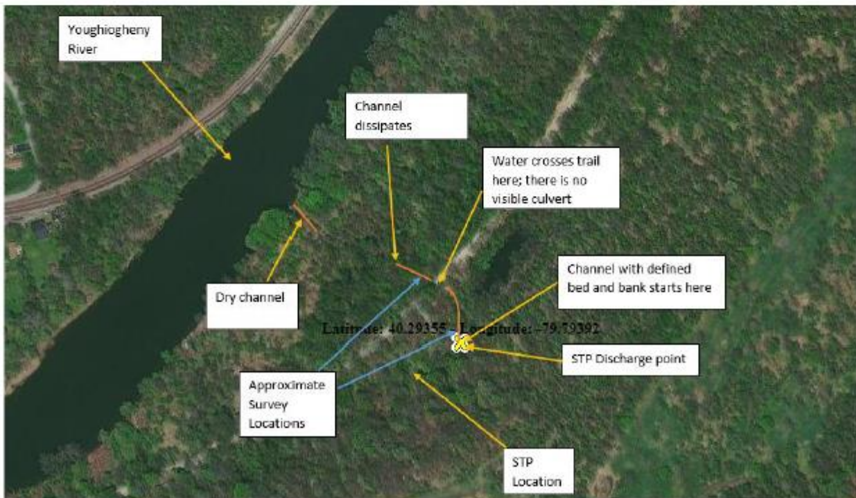
Figure 2. Aerial showing the location of the STP, the STP discharge, surveys, and the channel that carries the STP discharge toward the Youghiogheny River. Please note, locations are approximate.
