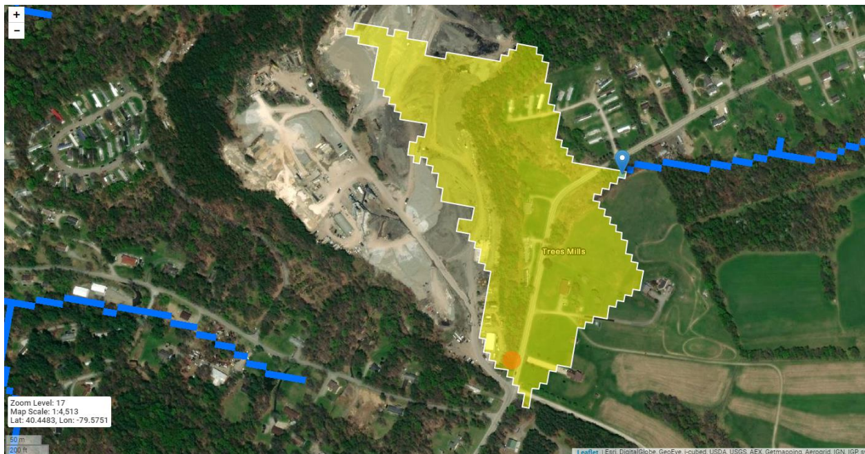
Figure 6: Drainage Area at the Headwaters of UNT 42998 of Beaver Run and Location of Outfall 004
