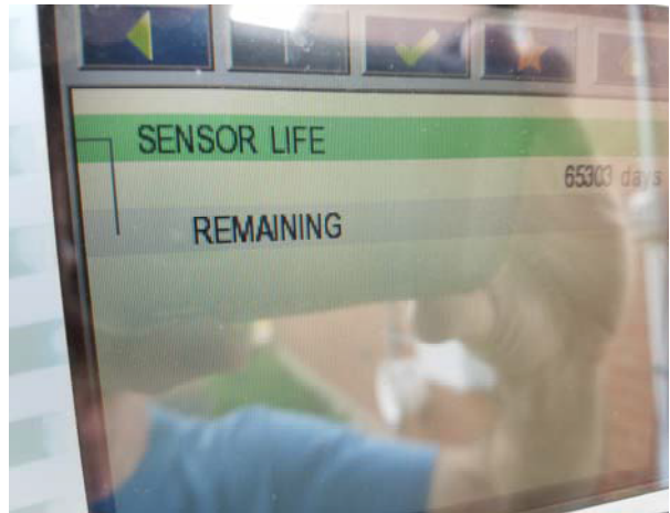
Sensor Life: 178 years or 7.45 years (if hrs not days used in the firmware)
