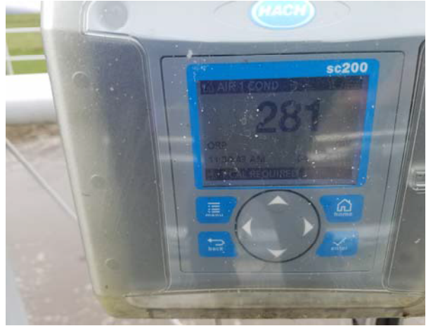
Controller notes probe recalibration is due
