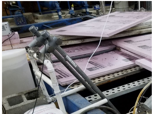
5-probe setup: pH and NO3-N
