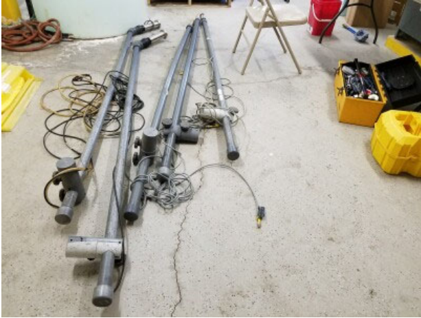
Monitoring probes during installation
