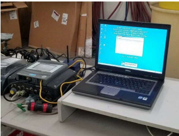
Data logging system and probe controller
