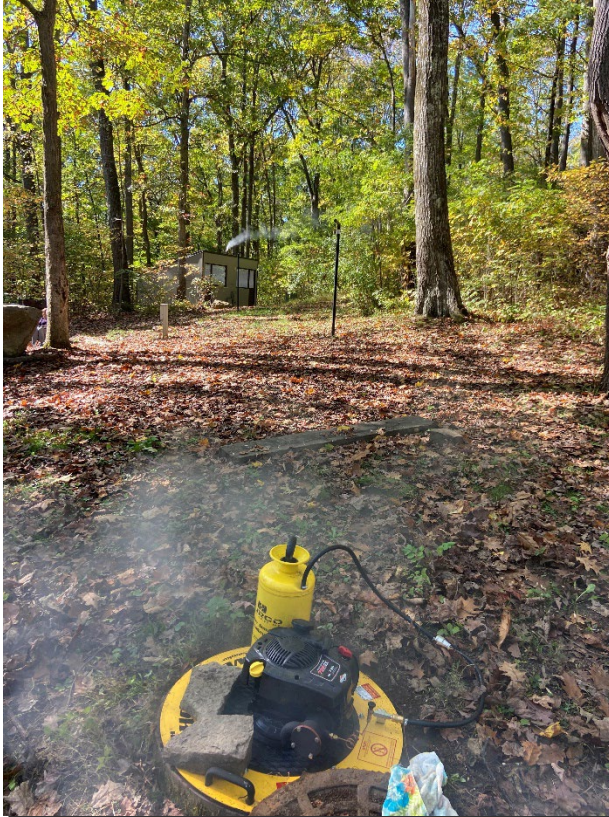
Smoke machine in process and smoke seen coming from building vent.
