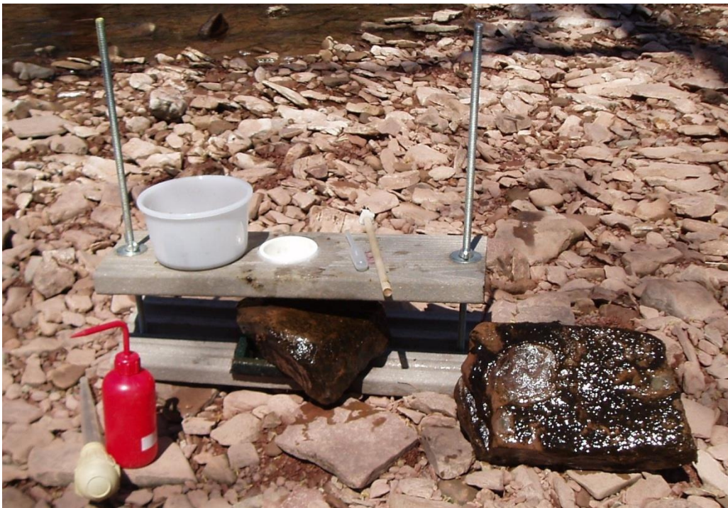
Figure 1. Pennsylvania Epilithic Periphyton Sampler.
