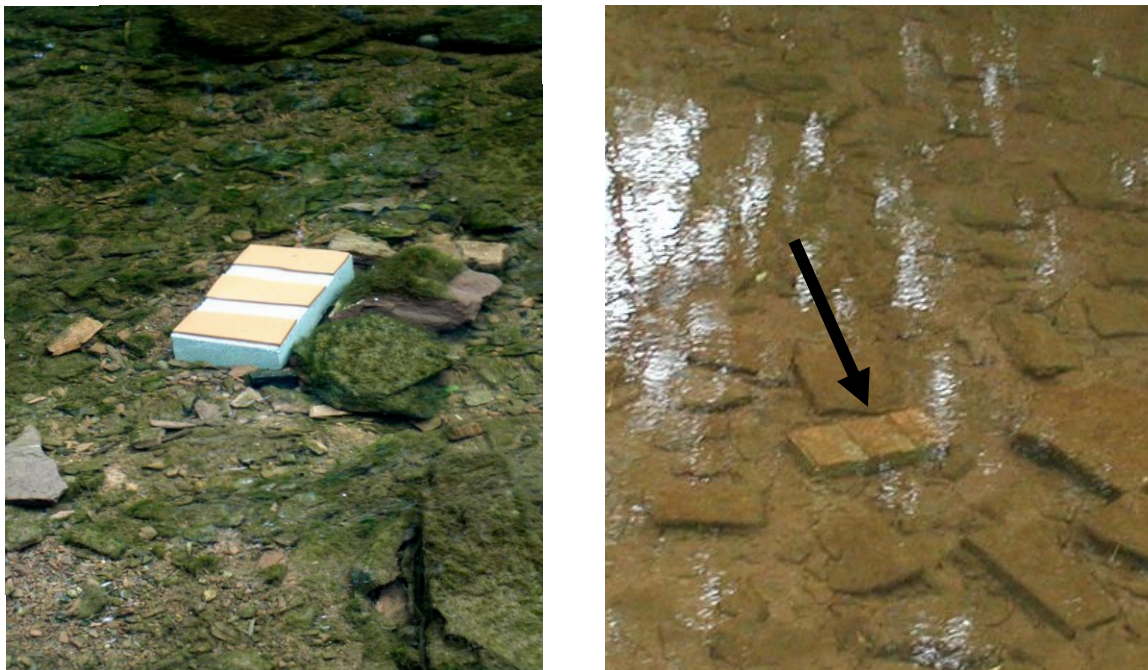
Figure 2. Example Clay tiles to be used as artificial substrate in Phase 2. Left photo taken day of deployment, right photo after 14 days growth
