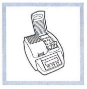
**6.** Insert the vial into the DRB200. Close the protective cover.
