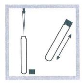
9. Use a TenSette Pipet to add 2 mL of 1.54 N Sodium Hydroxide Standard Solution to the vial. Cap and mix.
